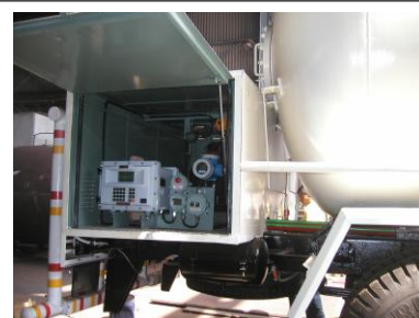
Meter with Batch Controller on LPG Truck
